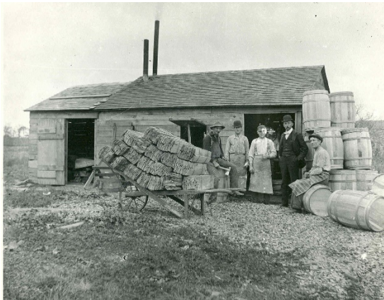
A cart of staves ready to be turned into barrels at cooper shop, Lockport NY
